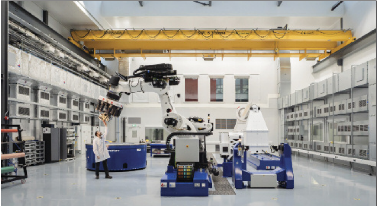
A cell for automated fibre-placement and automated tape-laying processes installed at the UK's National Composites Centre.
