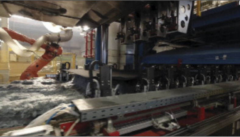
In a single step, Adler-Pelzer's hot-moulding process can make a floor carpet (HMPtex) with either a velour or tufted surface and an integrated backing for acoustic insulation.
