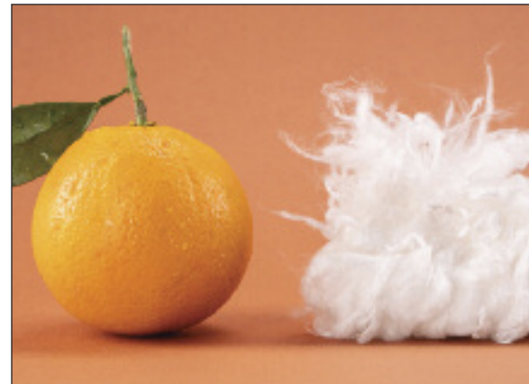
Tencel Limited Edition x Orange Fiber is manufactured from wood pulp and by-products of the processing of citrus fruit.
