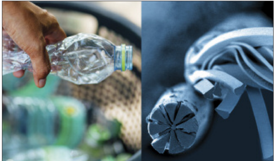
Freudenberg is using polyester sourced from post-consumer recycled plastic bottles (left) to produce Evolon microfilament textiles (right).
