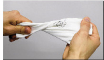
The flexible silk-based coil is shown here sewn into a textile, and is capable of harvesting energy from wireless internet and other radio waves present in its surrounding environment.
