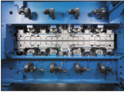
The infeed side of Dilo's double needleloom with blowing nozzles at the stitching plates.
